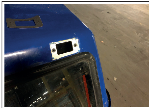
Figure 6 - Installation of new wellnut
