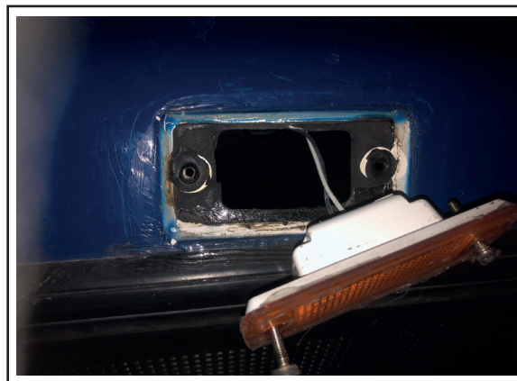
Figure 2 - Broken marker light
