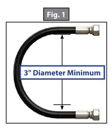
**NOTE:** If hoses need to be replaced, measure and make the hydraulic hoses. Always follow the manufacturer's specifications for the correct minimum bend radius throughout the entirety of the hose route. Use gauges to verify areas with questionably tight bends. Fitting orientation can be adjusted to achieve this in some applications. The correct bend radius is shown in Fig. 1.
