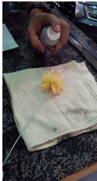
Figure 3. Applying all-purpose cleaner D 009 401 04 to the tip of a hummingbird feeder cleaning brush. The cleaning brush can alternatively be saturated with isopropyl alcohol.
