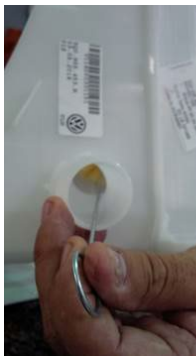
Figure 4. Cleaning the sensor probes.
