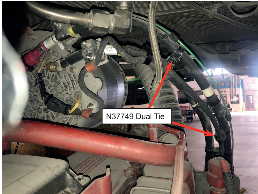
Figure 16 - Installation of Dual Clamp tie
