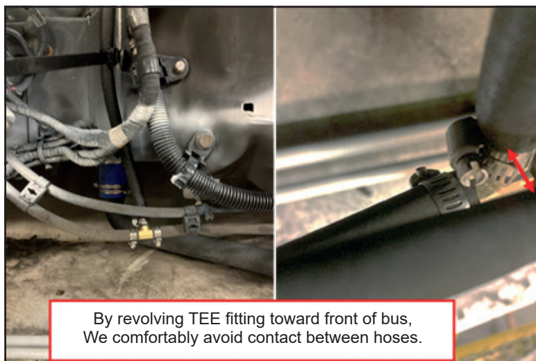
Figure 8 - Installation of Relief Valve Hose
