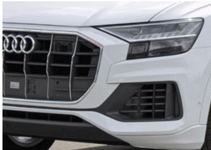
Figure 2. Correctly configured radiator grille trim in body color.
