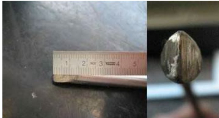
Figure 9. Ground the tip of the steel rod.
