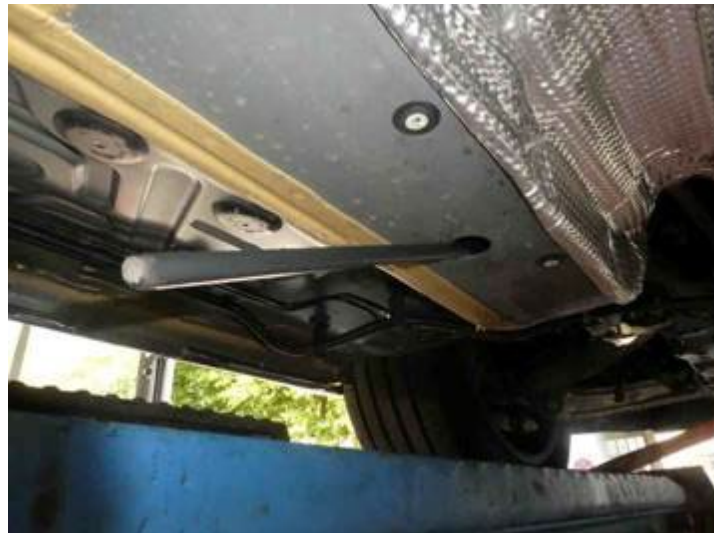
Figure 10. Insert the steel rod.
