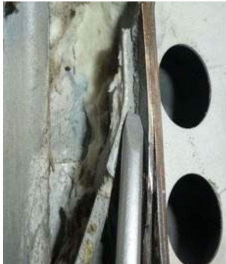
Figure 16. Incorrect engagement of the chisel end.
