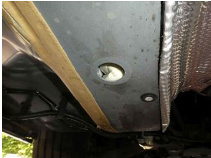
Figure 6. Body plug removed.
