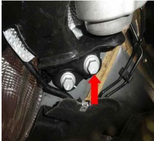
Figure 1. Front most bolt on subframe to be loosened.
