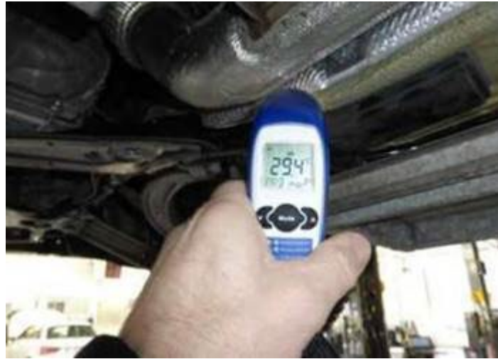
Figure 5. Surface temperature cooled to approximately 30° C (86°F).
