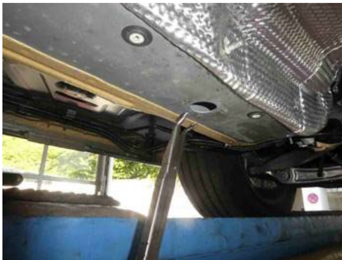
Figure 7. Remove a portion of the acoustic foam.
