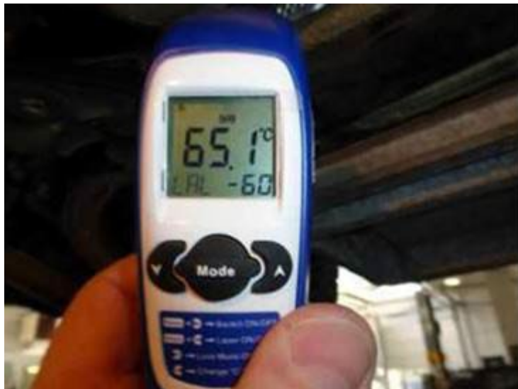
Figure 4. Surface temperature warmed to 65° C (149°F).
