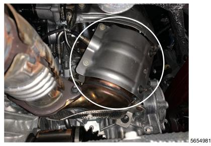
1. Inspect the catalytic converter part number. Refer to Catalytic Converter Heat Shield Replacement (Lower) to remove the shield for inspection.
