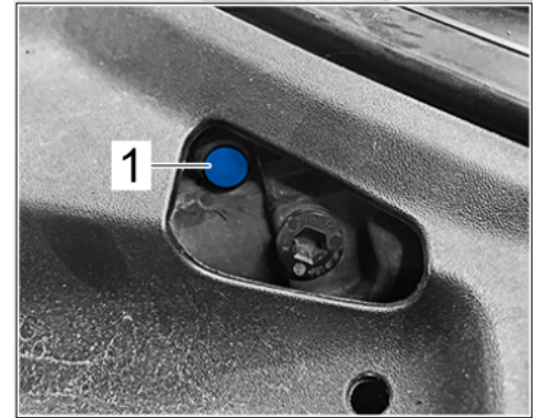
Installing locking cap (e.g. Cayenne MY 2016 left headlight)
