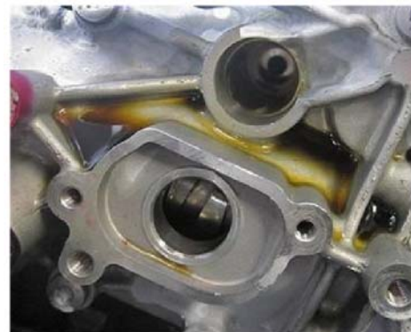
Fault type 2: Cylinder head cover leaking
