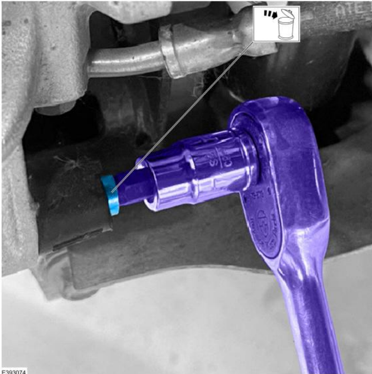
6. Rotate the rear caliper upwards to access to the bushing housing. (Figure 6, Callout 1) Figure 6
