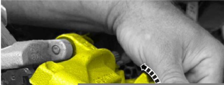
6. Rotate the rear caliper upwards to access to the bushing housing. (Figure 6, Callout 1) Figure 6
