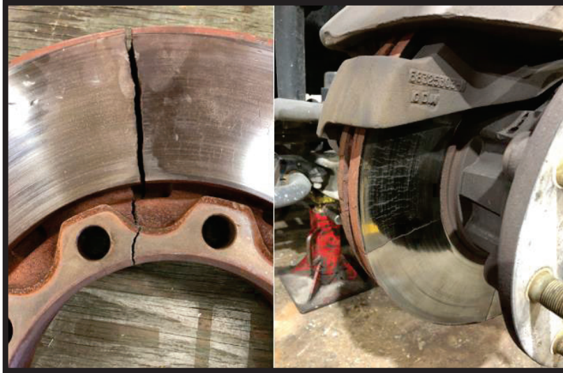
(Example of failed rotors)
