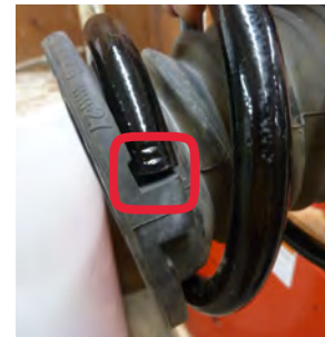
Lower end of coil spring at lower rubber seat
