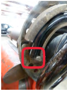
Upper end of coil spring at upper rubber seat
