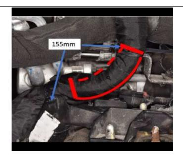
Install the updated Zip Tie style Fir Tree Clip GM PN 13596790 in the Generator Bracket as shown below.
