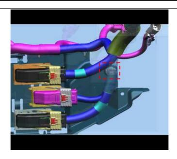
Protect the engine wiring harness from future damage at Generator Bracket. Zip Tie style Fir Tree Clips are located on the plastic Channel at #1 and on the Generator Bracket at #2 shown below
