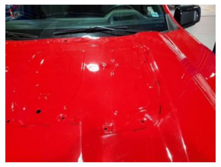
7. Next, using a combination of the different length pieces of tape, place them on the hood with the sticky side down against the paint following the hood indentation, as shown below. Place the tape with the outer tape edge 1 to 2mm from the edge of the hood indentation, as shown below. Along each side, stop the tape 10mm from the rear edge of the hood.
