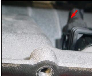
21. Confirm the O-ring is installed at the location shown.
