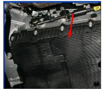
8. Remove 10 bolts that secure the valve body to the case and remove the valve body.
