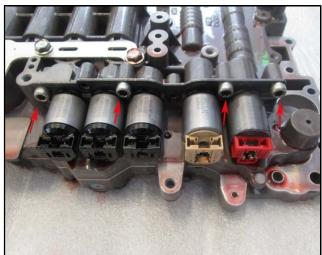
15. Pull out the related solenoid and install a new solenoid.
