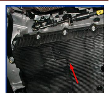
ATF TEMPERATURE = 122~140°F (50~60°C) SHIFT LEVER IN "P" AND ENGINE RUNNING
