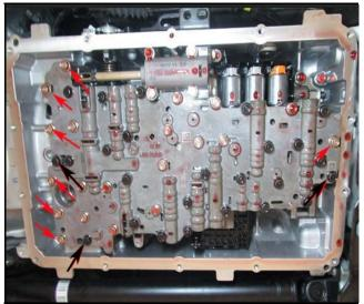
9. Remove 9 bolts and remove the E-module.
