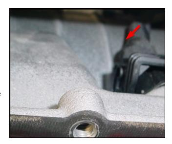
6. Use an 8mm or 5/16" hex wrench and remove the fill plug.
