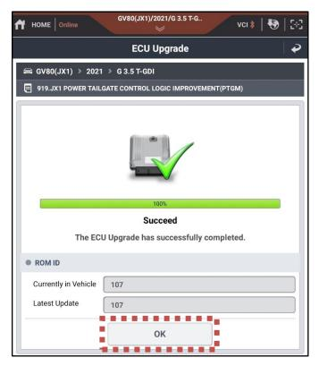
20. After upgrade, remove power connector of indoor fuse box, and reconnect it after 5 seconds.
