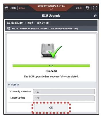
10. After upgrade, remove power connector of indoor fuse box, and reconnect it after 5 seconds.
