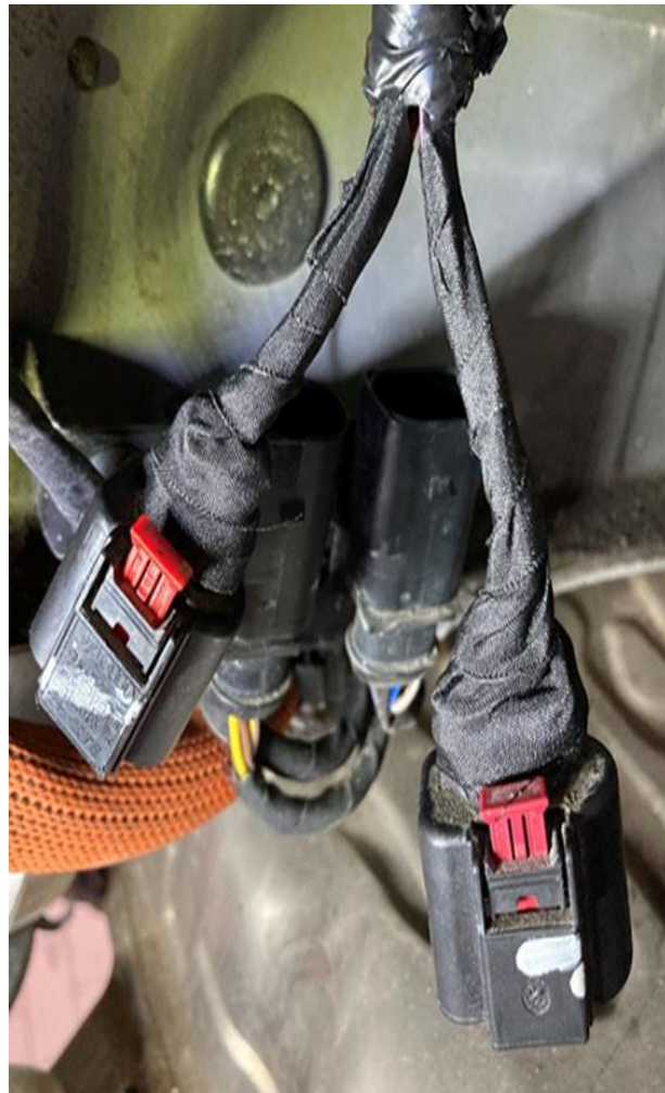
Figure 5: T6bl and T8bd harness wrapped.
