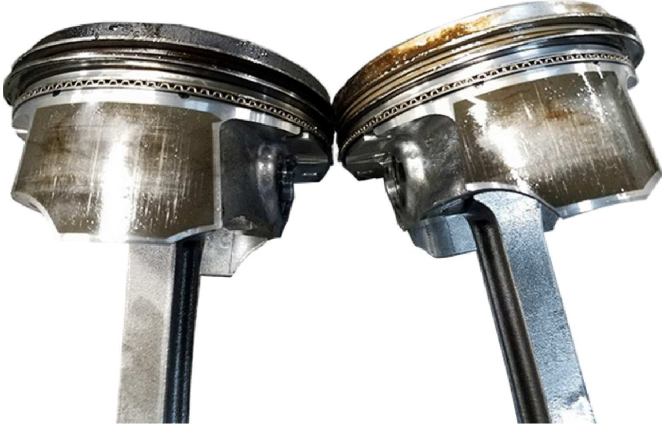
The piston skirt and piston ring damage caused by abrasive cleaning pads.
