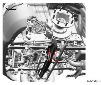
8. Remove and discard the U-bolt nuts (1) on the U-bolt that were over torqued.
