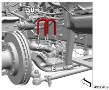
9. Remove and replace the U-bolt (1) that was over torqued.
