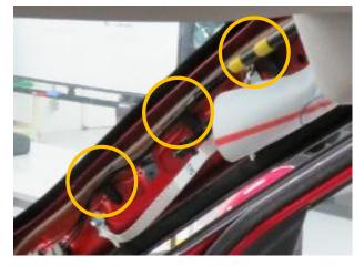
5. Reinstall the Front Speaker, Front Speaker Garnish, and Front Pillar Garnish. \*[CLIP, FR PILLAR TRIM (Part No. 7210A329)] is non-reusable parts.
