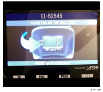
2. From the Fob/Key ID screen, the tool will instruct to place the fob on the small pocket on the back of the tool and press OK.
