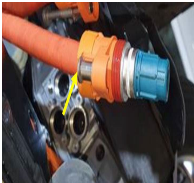
Figure 2: Connector end at the power electronics module.
