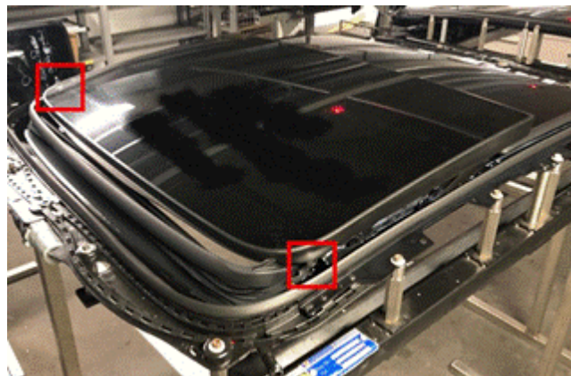
Figure 2. Front sunroof glass panel side skirt protrusion from an unmodified water guidance washer.
