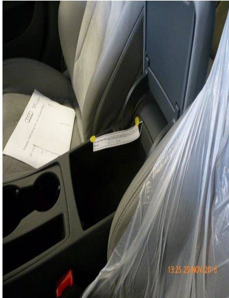
Figure 1. The first photo should show a full picture of the affected component and the affected area of the cause should be marked with an arrow (paper with yellow dots). This is for guidance.
