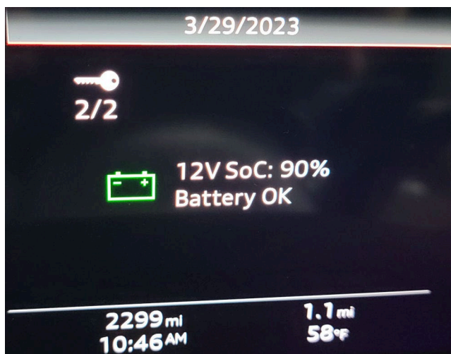
Figure 2: SoC display in transport mode.
