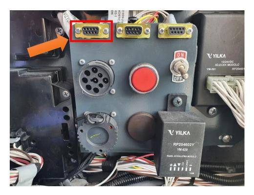
3- Connect one end of the KIBES cable to the CANalyzer or Peak cable and the other end to the KIBES diagnostic socket. Connect the CANalyzer or Peak output to the computer. Make sure that the KIBES dongle is inserted to your computer.
