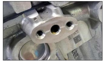
Perform the polishing procedure on the RH side according to steps 5 - 15 of the TURBOCHARGER OIL FEED REWORK (LH SIDE) procedure.
