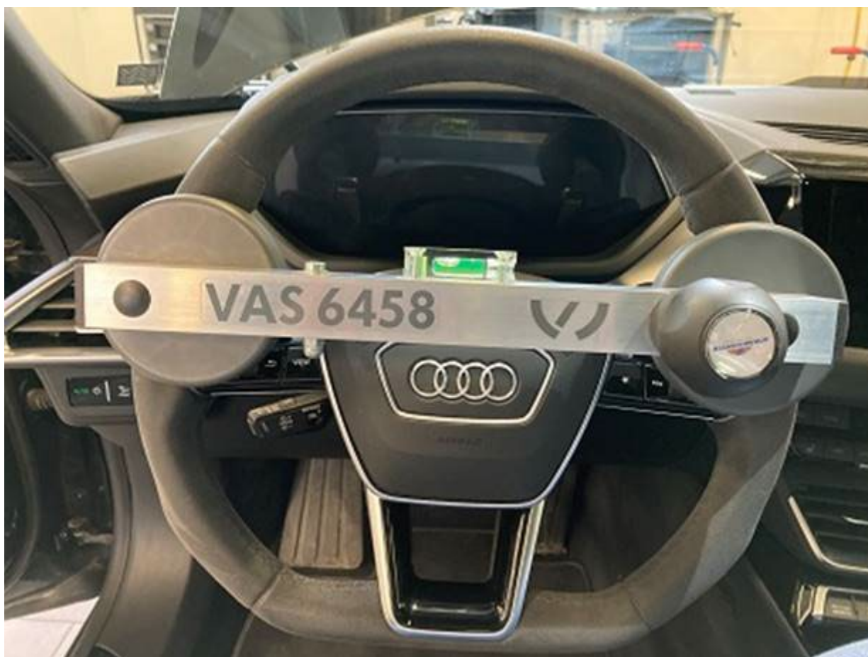
Figures 1 to 5: Examples of Steering wheel off center by 2° to the left and 2° to the right with VAS 6458 and VAS 6826 installed.
