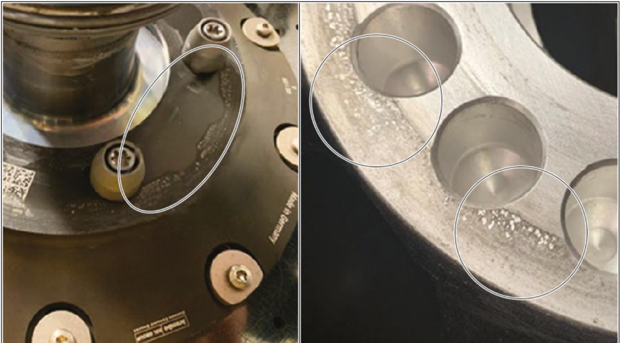
Material transfer for brake disc/wheel hub
