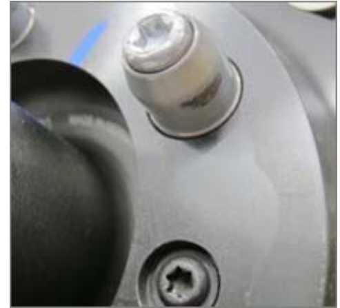
Material transfer on driving pin
