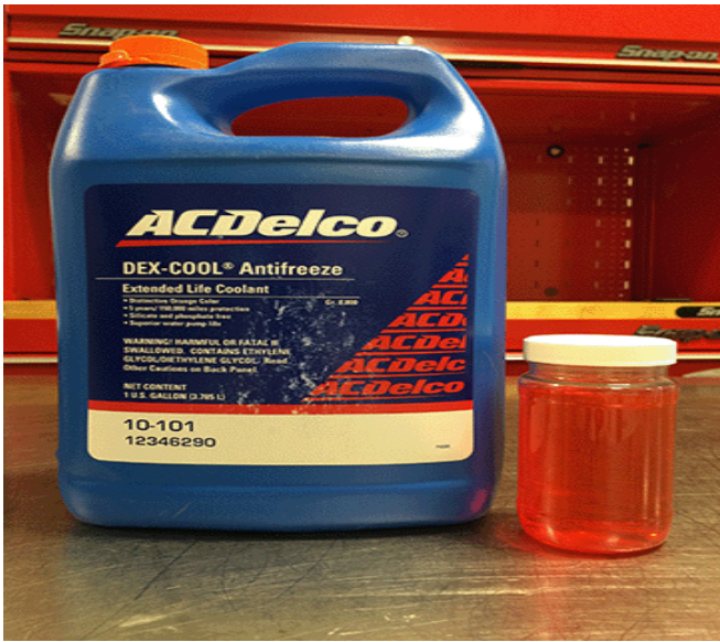
Diesel Exhaust Fluid (DEF) mixed with Dexcool.
