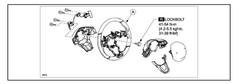
**NOTE:** For vehicles with a steering wheel warmer, replace the steering wheel hub kit (A).
