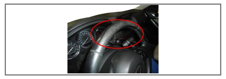
**NOTE:** Slight wear on a seam of the steering wheel is not applicable to this bulletin. It is inevitable since friction and force are applied while turning the steering wheel.
