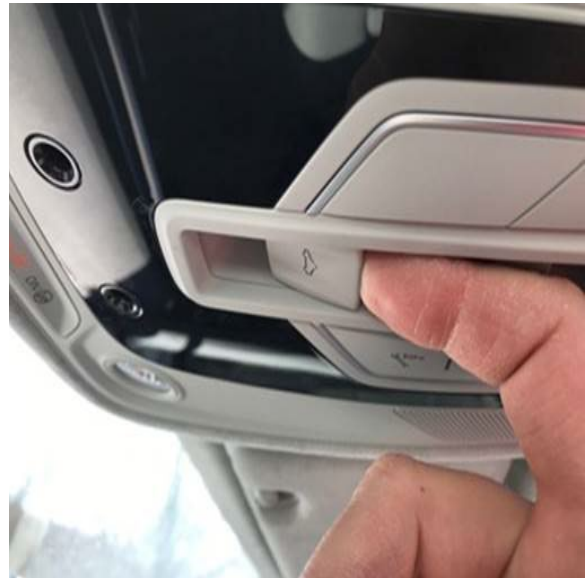
Figure 1. Set the sunroof panel basic settings by pulling the sunroof switch fully downward.
