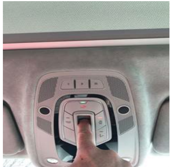
Figure 2. Set the sunroof shade basic settings by pushing the sunroof shade switch fully forward.
