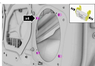
b. In 4 locations: Using the special tool: Install:
