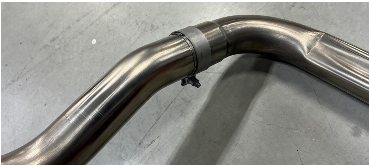
Figure 6 – Fleet Value Catalytic Converter Slip Joint (Off Vehicle)
