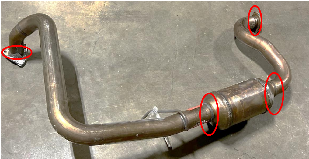
Figure 8. - OEM Catalytic Converter Assembly (4 pipe welds)
