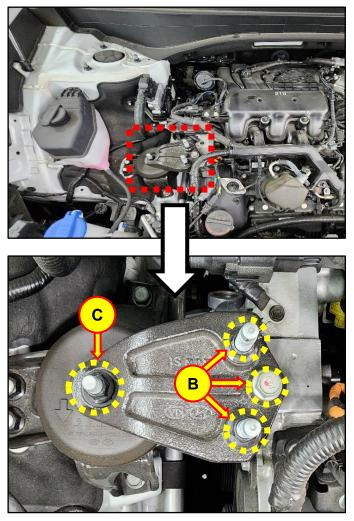
3. Take a STUI photo of the 4 retightened engine mounting support bracket fasteners.
