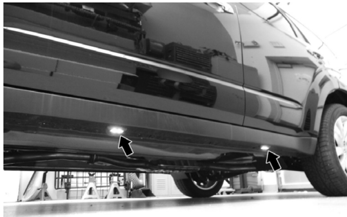
CHECK FOR FUNCTIONING PUDDLE LIGHTS
