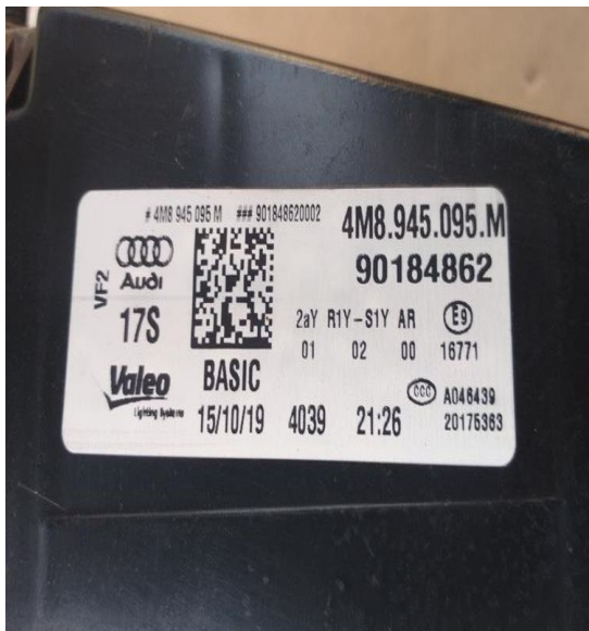
Figure 5. Example of tail light assembly label.
