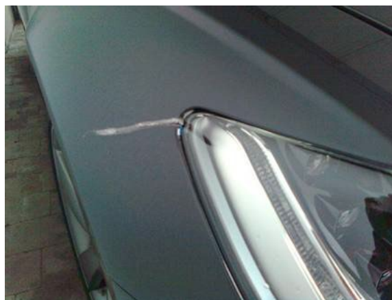
Figure 1. Car wash bristle is stuck in the body gap.
