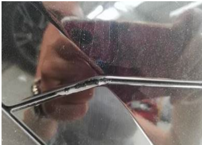
Figure 4. Moderate loss of adhesion.
