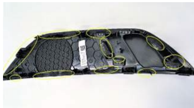
Figure 2. All tabs on the midrange speaker trim that require felt tape.
