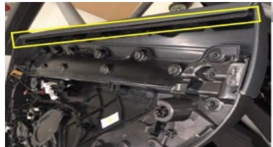
Figure 4. Fleece tape applied to mounting strip.
