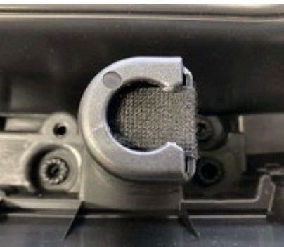
Figure 6. Door clip with fleece tape applied.
