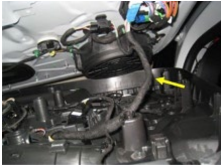
Figure 12. Wire harness not secured properly.
