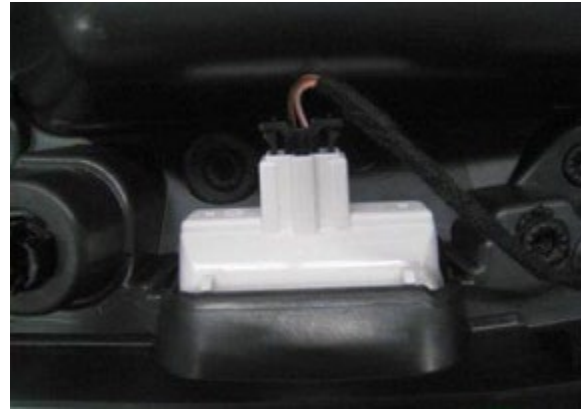
Figure 17. Wrapping light wire harness with fleece tape.
