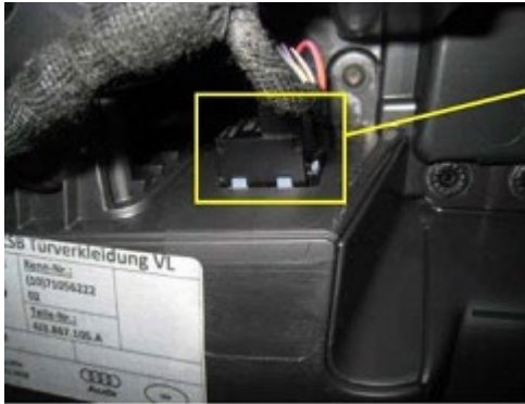
Figure 21. Apply fleece tape to pocket lighting.
