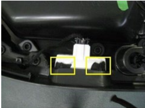
Figure 18. Fleece tape applied to light assembly.
