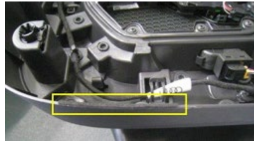
Figure 15. Felt tape installed on trim panel.
