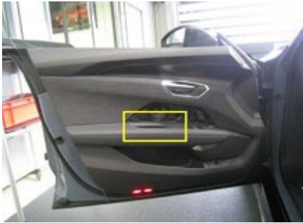
Figure 8. Isolate pull handle from armrest.
