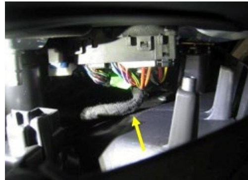
Figure 11. Wire harness contacting door trim panel.
