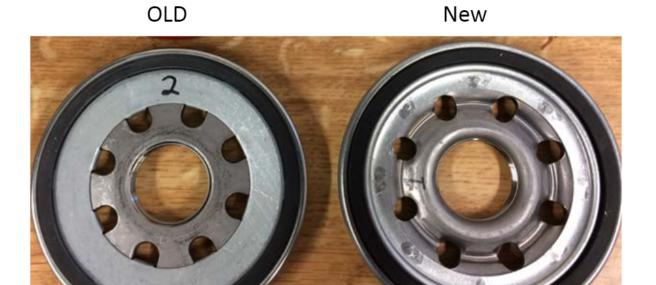
Volvo 21879886 Shallow Groovewill not fit on the US2017 fuel filter housing
