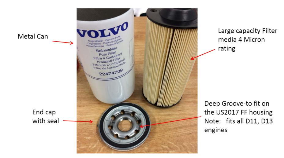
US2017 engines use New Primary and secondary engine fuel filters
