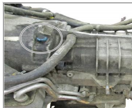
Oil loss from PDK vent
