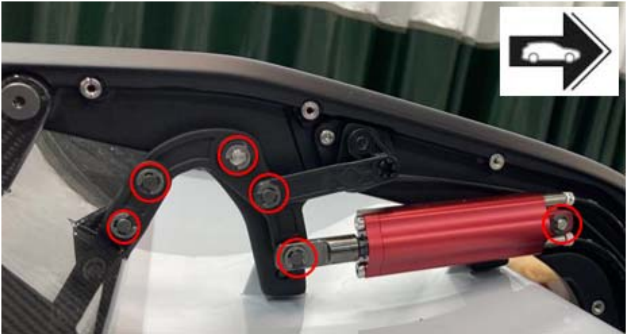
Circlip installation positions - left wing strut shown
