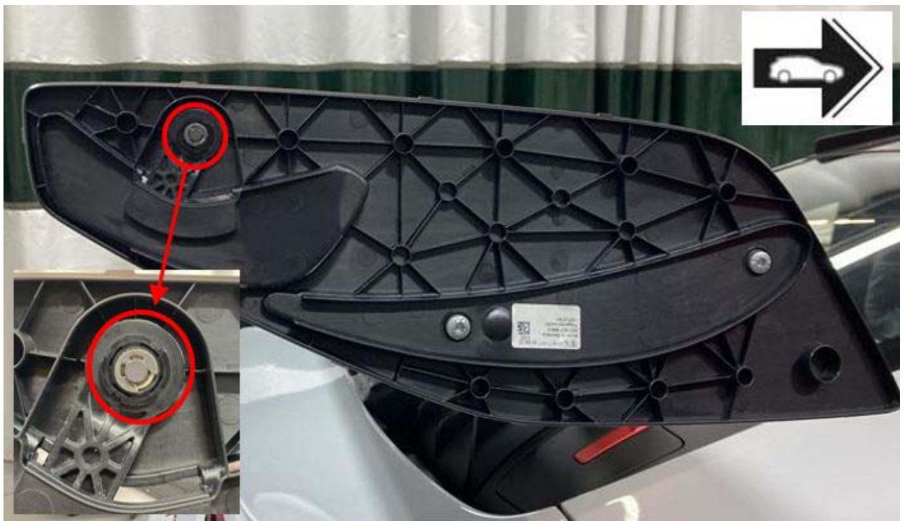
Circlip installation position - right side cover shown
