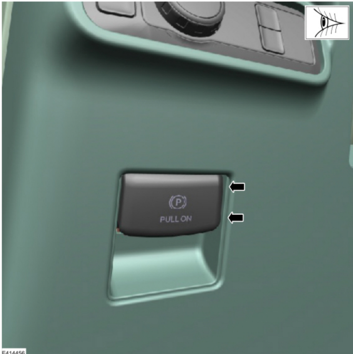
Figure 2 - Pull-down Style Parking Brake Switch
