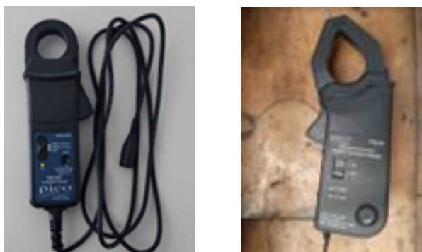
Figure 9: current clamps to be used for the measurement of current absorbed by the compressor.
