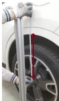
Figure 3: measuring method of the Vehicle Height at each corner.
