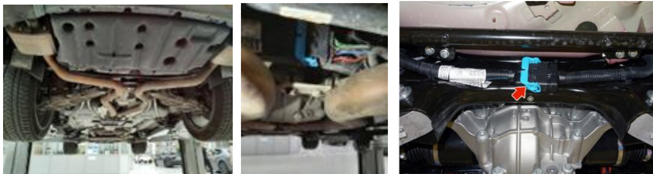
Figure 7: position of the X090 connector for the current measurement absorbed by the compressor during the actuations. And secondary lock (blue, indicated by the arrow) of the X090 connector
