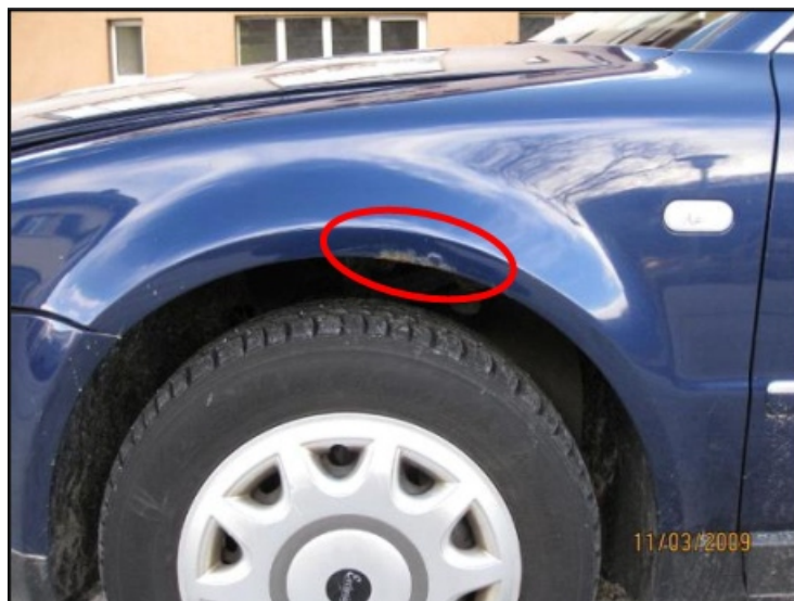
Figure 1 (corrosion on left wheel arch)
