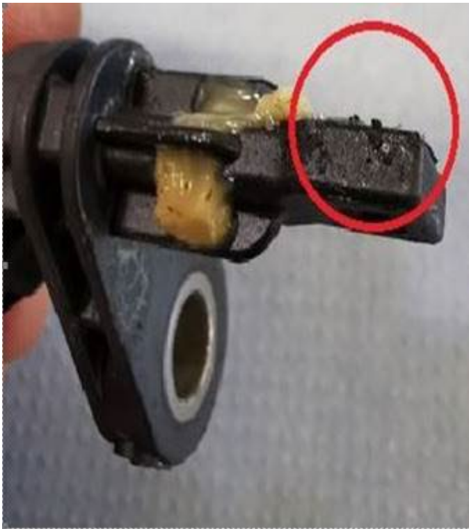
Figure 2: Metallic particles in the speed sensor.
