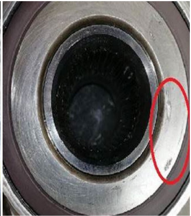
Figure 5: Metallic particles/damage in the wheel hub/bearing.
