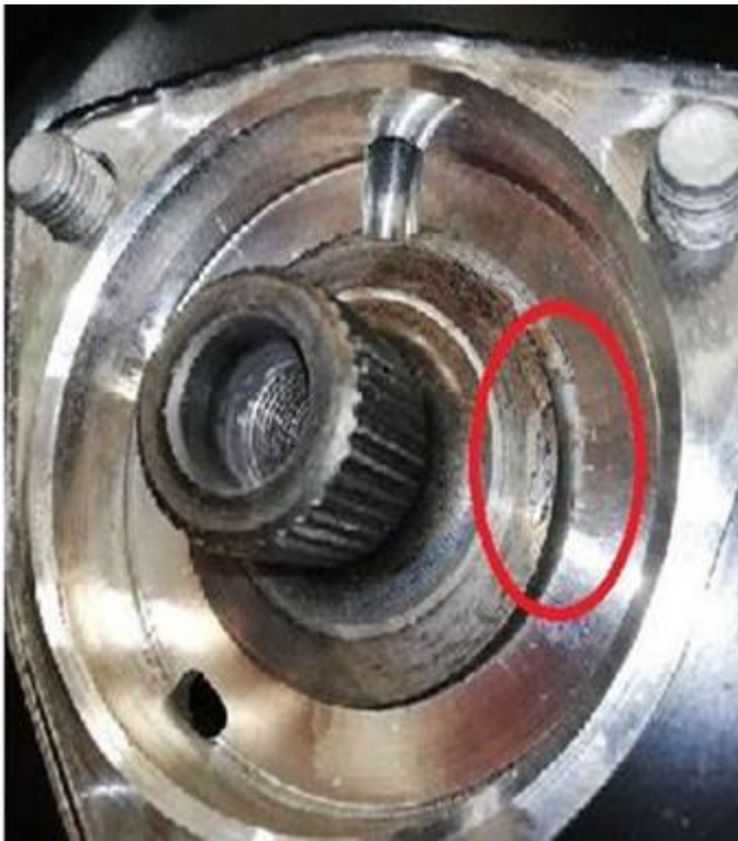
Figure 4: Metallic particles/damage in the wheel hub/bearing.
