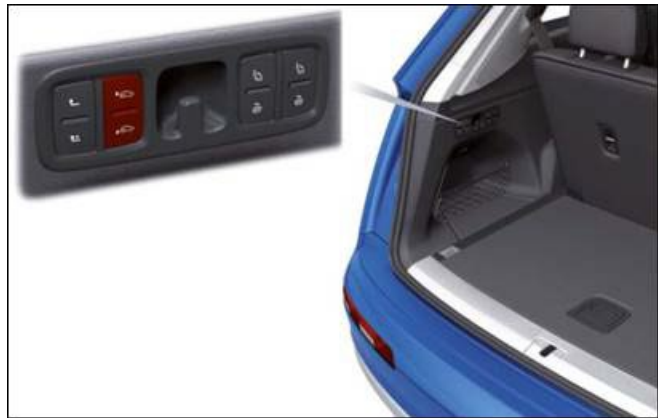
Figure 1. Location of the controls for lowering the rear suspension.
