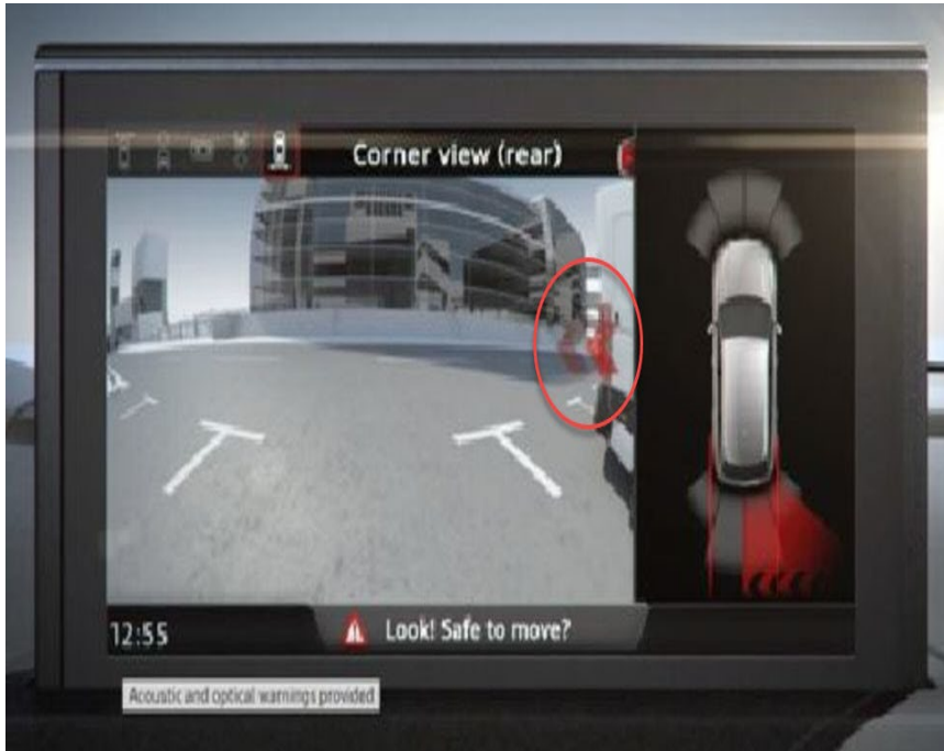
Figure 1: RCTA/Intersection assist arrows.
